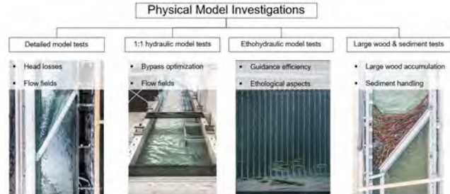
Fig. 3: Different model setups to optimize the design of FGS and bypass and maximize the FGE
