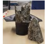
Figure 1b: Tested sample under 200 MPa and 200°C.
