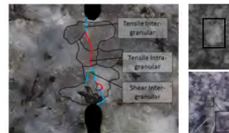
Fig. 5: Type of cracks and grain boundaries (left). White patching: extended zone (top right) and punctual (bottom right) in hydroshearing experiments.
