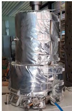
Figure 2: High PT triaxial device with heating jacket.
