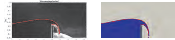
Fig. 4: Qualitative comparison of water surface between the experimental and the numerical data. Initial parameters are: h = 0.25 m; a = 0.075 m; b_c = 0.02 m; w = 0.30 m.
