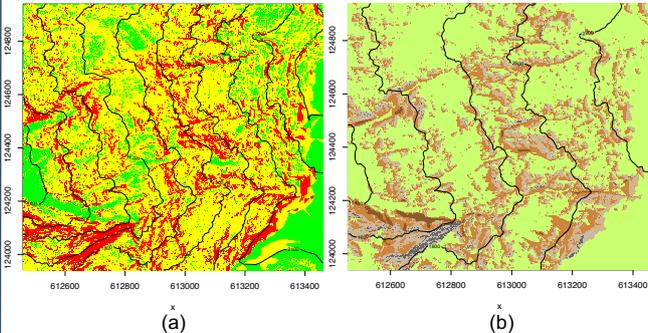
Fig. 2 : (a) The factor of safety (FS) contour map before the application of LSgCA, red patches indicating the unstable cells (FS  $\leq 1$ ). (b) Propagated landslide after the application of LSgCA; brown patches represent the landslide thickness; Scarps are shown in dark grey color.
