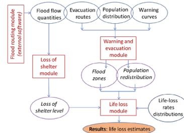
Fig. 3 HEC-LIFESim approach for LL estimation (modified from Bowles, 2007)
