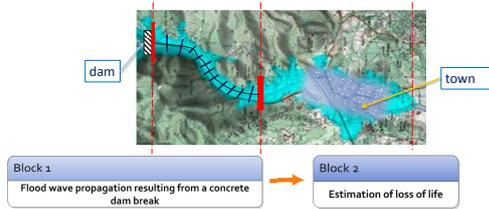
Fig. 1. Essential computational blocks for the modeling of the dam-break event
