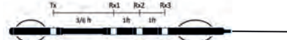
Fig.1: Sonic log tool with one transmitter (Tx) and three receivers (Rx1, Rx2, Rx3).
