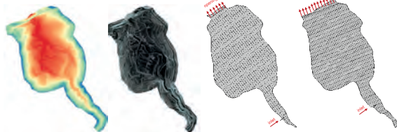
Fig. 2 – From the left to the right: Qgis DEM, contour lines, Rhino geometry 1753 m a.s.l. and 1767 m a.s.l.
