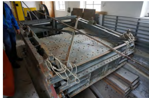
Fig 4: Rail wagon with a weight of approx. 6 tons. Additional weight will be added with steel plates and water tanks. The wagon front will be equipped with a vertical steel plate to increase momentum transfer.
