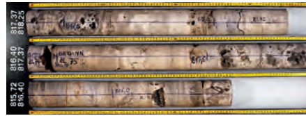
Fig. 2: Drill-core section of the Trigonodus Dolomit at the BEN borehole. The cm-dm scale cavities originate from the dissolution of eogenetic anhydrite nodules.
