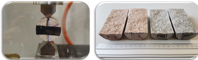
Fig. 1 Left: Brazilian induced fracture and Right: comparison of thermally shocked (left) and not shocked (right) samples.
