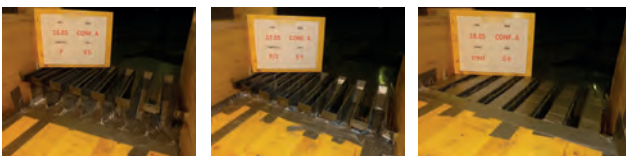
Figure 4: Rating curves tests: fixed level at P (left), at P/2 (middle) and at the crest (right)
