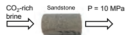
Fig.1 Sketch of the model with constant flow rate at the inlet and constant pressure at the outlet.
