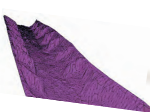
Figure 1: Resulting mesh from grain field with a DTM recording with a vertical exaggeration factor of 3; 3D mesh representation done with Basement (dry bed).
