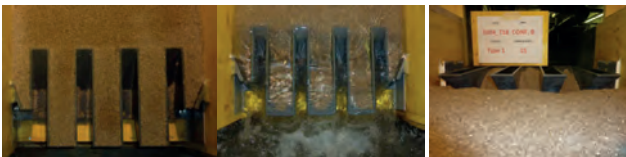
Figure 3: Test 18 - Starting conditions (left), during test (middle) and final conditions (right)
