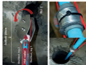
Figure. Measurement setup for A-DTS tests in INJ 1 and INJ 2 boreholes. The bottom-piece and the connection points of the DTS / injection rod. The cable connection points were isolated towards the injection tube with pieces of foam.
