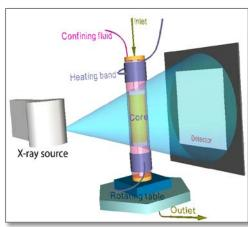
Before and after reaction XRCT imaging + Radon Transform for volume registration
