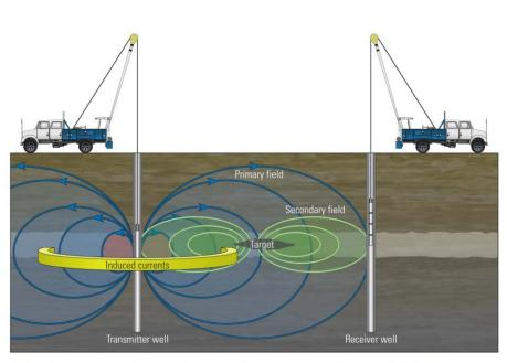
**Fig. 4**: Basic setup and principle of crosswell EM (Oilfield review summer 2009, 21, no. 2. Schlumberger).
